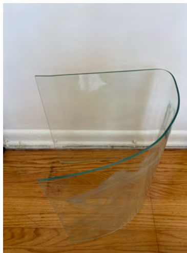
Fig. 36 (Acrylic after bending)
